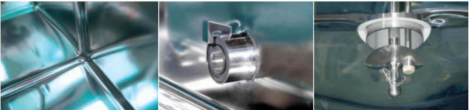
Internal cleaning via high-performance rotating spray head with rotation control
